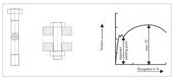
Tensile test on a turned-off screw Fig. A Tensile test on a whole screw Fig. B
